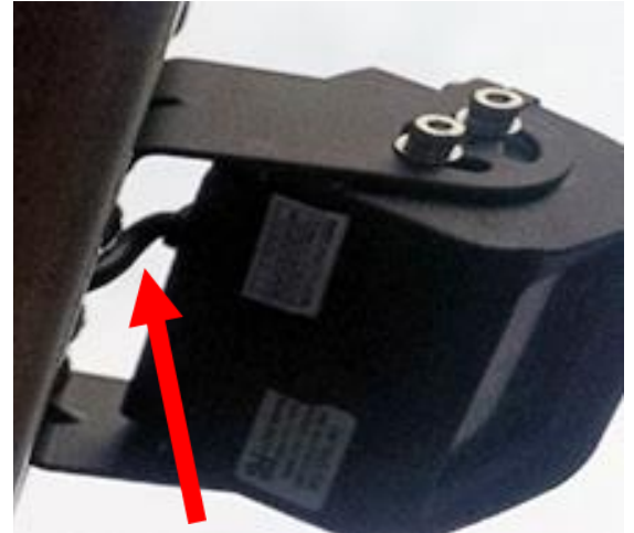
Too Much Cable Tension
